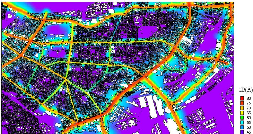
Figure 7 Contour Map when HV is ban along highway route (A  $\leftrightarrow$  B) (CASE-1)
