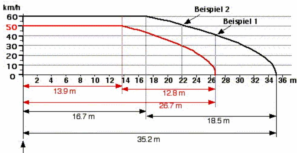
Example 1 (Beispiel1): At the point, where the vehicle with the speed of 50 km/h at the beginning of the breaking manoeuvre is brought to a stop (26.7 m) the collision speed of an other vehicle with a beginning speed of 60 km/h is still 40 km/h.
