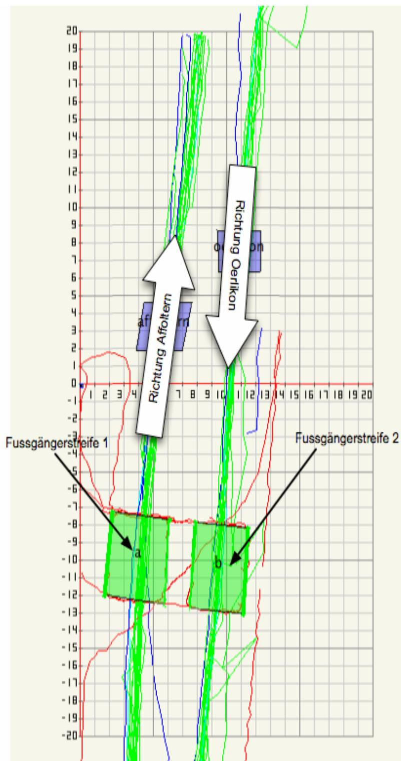
The illustration shows the installation of the laser-sensor at a pedestrian-crossing (green rectangles). The cars are green lines, the bicycles are blue lines, and the trucks (or buses) are light blue. The red line shows the pedestrian who was marking the site of the pedestrian crossing with central island.
