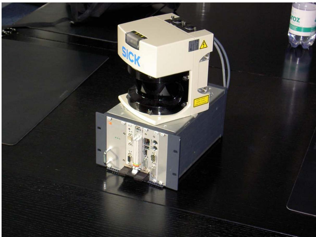
The components of LOTraffic: Laser sensor and industrial computer
