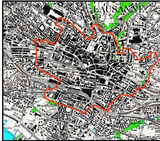
The simulated area, shown by Figure 3, includes 524 links and 241 nodes. Among the latter ones, 49 are controlled by traffic signals. Even if, in reality, the control plans are actuated, fixed plan have been simulated because no interface was ready for the integration of the VS-Plus [22] plans. The traffic demand is represented by a 80 per 80 OD matrix and the simulation period runs from 15h00 to 20h00. During the peak hour, a 16'500 veh/hour flow is recorded on the network.
