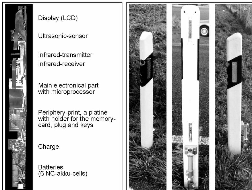
The speed of the vehicle is determined by analyzing the measured pass-through times in relation to the distances between the measuring poles. Each pole stores the collected data on memory cards, which are subsequently exported to a computer for further analysis.
