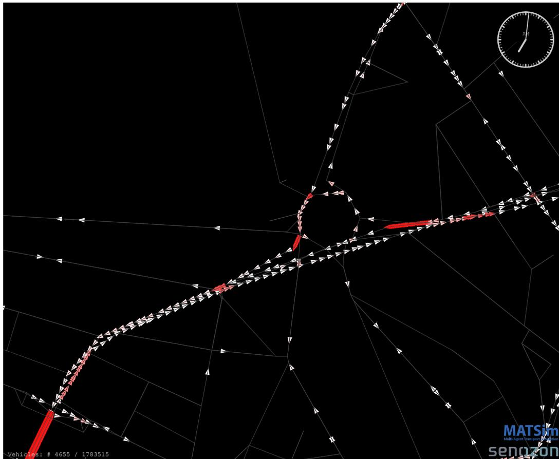
Some count stations indicate a dramatic situation, thus, the spatial characteristics of the jam are analyzed as well. Figure 5 shows that measured volume reduction does not cover the complete inner-city but is relatively limited to the wider neighborhood of the tunnels.
