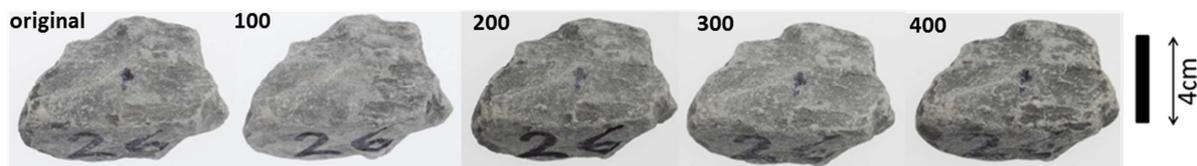
Figure 10 Roundness increase for some grains tested through the revolution stages.
