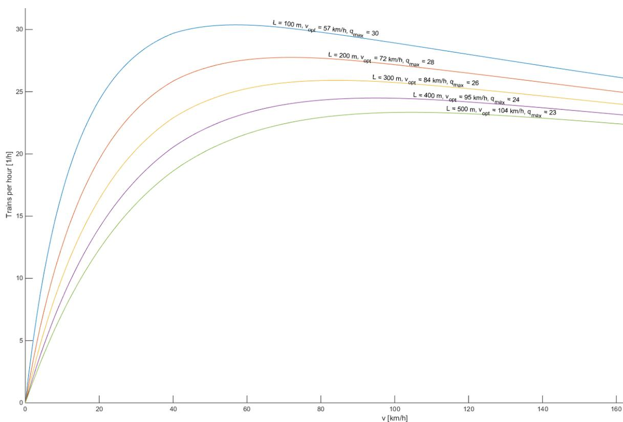
Figure 8 Maximum station capacity for automated trains
