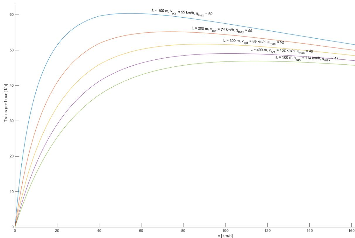
Figure 6 Maximum line capacity for automated trains
