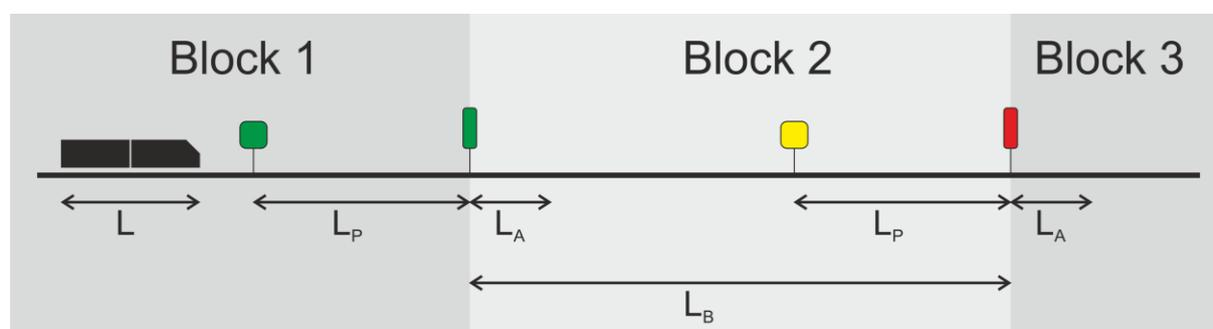
$L$  is the length of the train.  $L_B$  is length of the section block.  $L_P$  is the distance between the advance signal and the main signal.  $L_A$  is the overlap.
