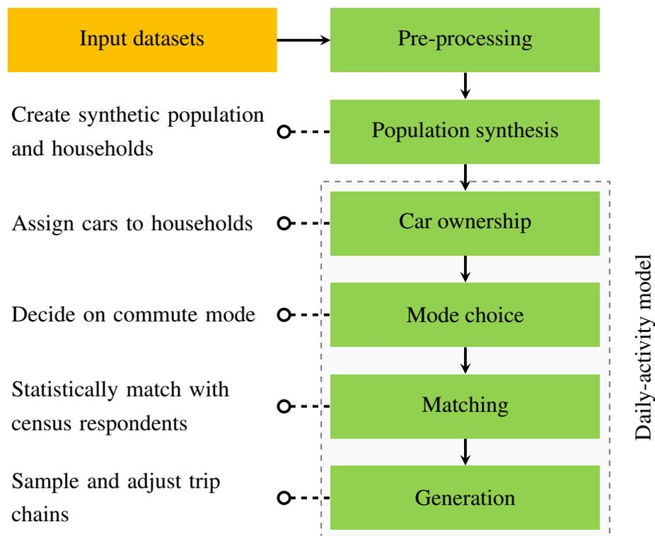
Figure 1: Structure of the main modelling pipeline.
