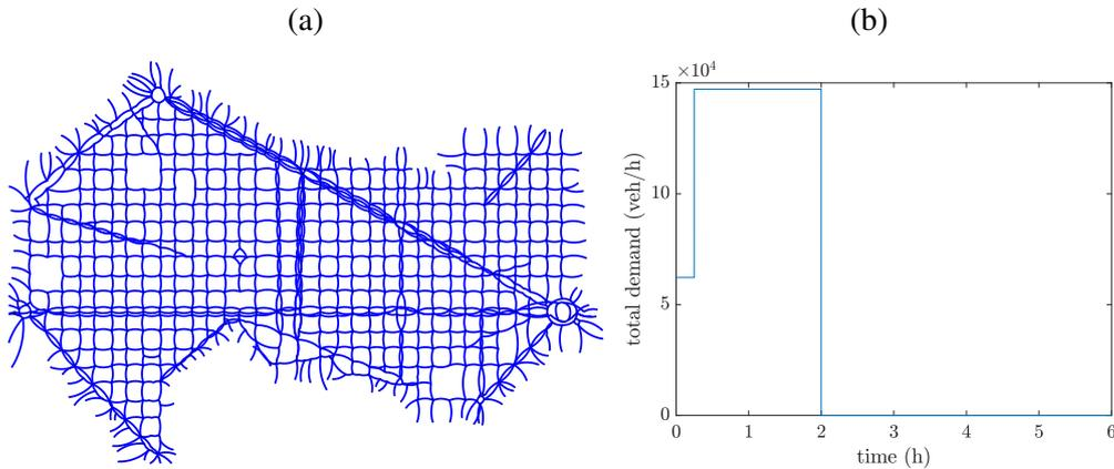
By performing all calculations described by the equations of the model for a number of time steps, we get a complete traffic simulation for the specific demand scenario. By knowing the queues of every link of the network at every discrete time-step (state variables  $m_z$  and  $w_z$ ,  $\forall z \in Z$ ), we can calculate the total travel time of all vehicles together with other traffic performance measures, as we will see below.
