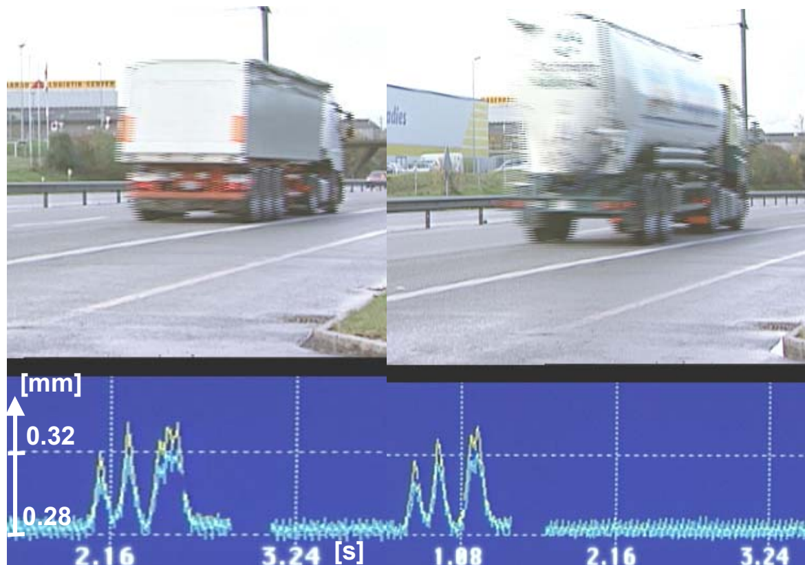
Figure 6 Vertical road deformations due to a passing truck, DDM device D2 in point 2B and 2D on the morning of 5th November 2002
