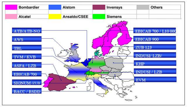
Figure 1: Different ATW/ATP/ATC systems through Europe
