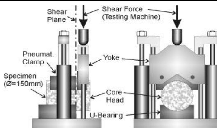
Figure 10 LPDS shear strength between porous asphalt and base course. Tests at EMPA.
