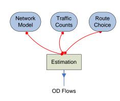
Based on this statement, this paper is going to analyze actual methodologies and propose an innovative approach particularly adapted for dynamic urban networks. This method is going to use traffic simulation (mesoscopic) for traffic assignment in the network (Route Choice in Figure 1).
