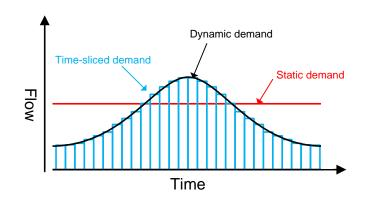
Figure 3 shows the different ways to represent traffic demand. Real and continue dynamic demand is represented in black. From this curve, traffic volume could be modeled by a time sliced approximation, in blue or in a very simplistic way, using a constant (static) demand during the whole period (in red).
