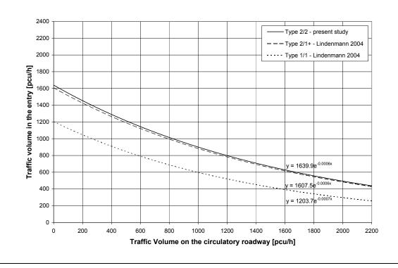
Figure 10 Comparison of the entry capacity of different roundabout types
