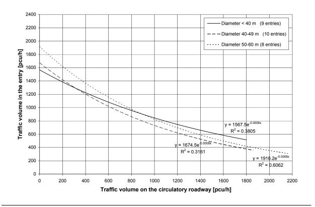
In case of low traffic volumes on the circulatory roadway the largest entry capacity results, as expected, for the roundabouts with large diameter. But in heavy traffic volumes on the circulatory roadway the entry capacity of small roundabouts (diameter < 40 m) is higher than the capacity of large roundabouts.
