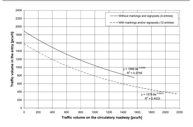
Figure 6 shows the unexpected result of the analysis of the influence of signposts and direction-indicating pavement markings on the entry capacity. Compared to scenarios with
