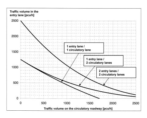
With the formula of the German Highway capacity manual (HBS, 2001) the entry capacity at a two-lane roundabout is much higher than at a one-lane roundabout. But it is assumed that in reality the influence of the second entry lane isn't that high because both lanes are rarely used equally.
